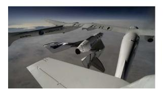
Figure 1: SpaceShipTwo release from WhiteKnightTwo
