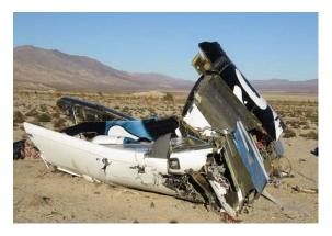
Figure 5: SpaceShipTwo Wreckage
