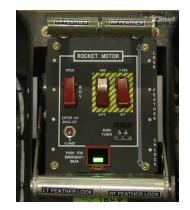
Figure 4: Feather Lock Handle - Unlocked Position
